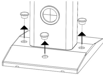
2. Place the Kiosk onto the Stabilization Base so that the holes line up as shown.
