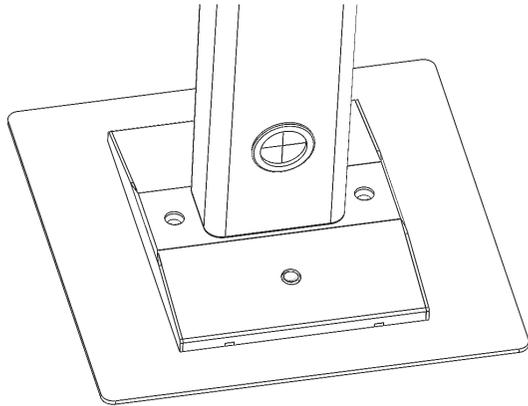
3. Screw the Kiosk to the Stabilization Base using the (3) M10 Socket Head screws and M10 Spacers provided.
