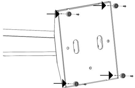
1. Remove the rubber plugs from the Kiosk as shown.
