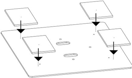
\*Remove the current Kiosk feet from the bottom of the Kiosk as shown.
