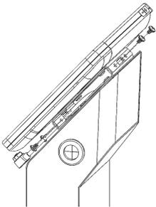
1. Install the 4 10-16 x 1/4 pan head self-tapping sheetmetal screws to screw the two Plates together.
