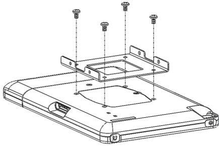
1. Install Plate onto CONNECT using the 4 10-32 x 1/4 pan head screws provided.
