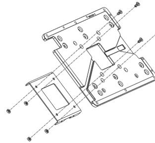
1. Install Plate onto PRO using the 4 10-32 x 3/8 pan head screws provided.
