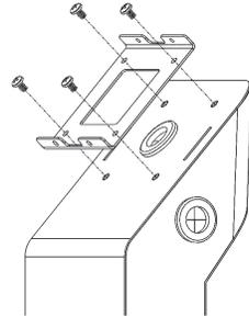
1. Install plate onto KIOSK using the 4 10-32 x 1/4 pan head screws provided.
