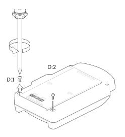
Open the Reader Cartridge, unplug the Moby/5500, and remove the card reader.
