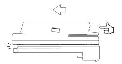
Pull the Reader Cartridge straight up to release.
