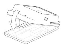
Tighten the Screws (D:1) into the Cartridge Bottom (D:2).
