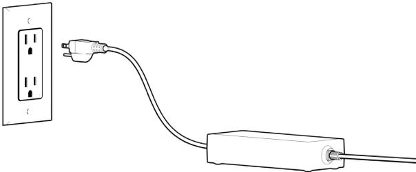
Plug the PDU into a wall outlet
