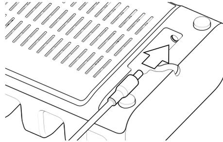
Plug the barrel connector into the Station
