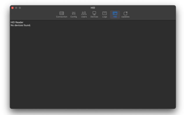
The HID tab is not visible by default, but can be enabled for troubleshooting on the Config tab.
